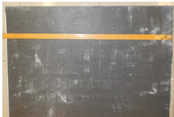
Figure 3: Bailey Interiors Slotted Perforated Plaster Ceiling Tiles with Sobertextile P44FR acoustic fabric installed in Reverberation Room.
