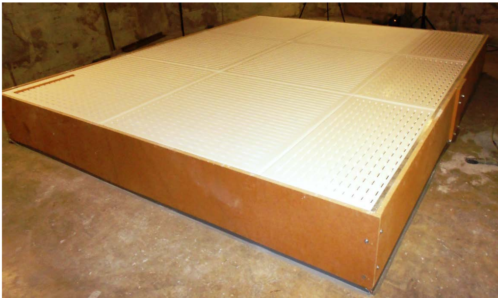
Figure 3: Bailey Interiors Slotted Perforated Plaster Ceiling Tiles with Sobertextile P44FR acoustic fabric installed in Reverberation Room.
