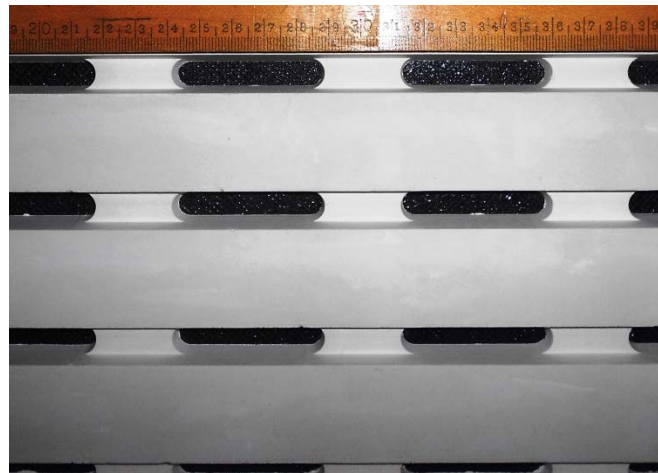
Figure 2: Rear Face of Ceiling Tile: Bailey Interiors Slotted Perforated Plaster Ceiling Tiles with Sobertextile P44FR acoustic fabric installed to rear of the tile.
